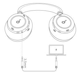
Play audio on an external device by plugging in a 3.5mm AUX cable. Wired listening will automatically turn off Bluetooth mode.
