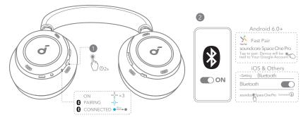
**Auto Pairing:** Press and hold the power button for 2 seconds to power on. The headphones will automatically enter Bluetooth pairing mode when connecting for the first time. Select **"soundcore Space One Pro"** on your device's Bluetooth list to connect.
