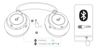
The headphones can connect with two devices at the same time. When already connected to one device, press the power button twice to pair with another device.
